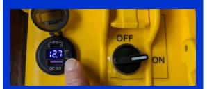
Turn on all units (2, 3 or 4) and check voltage on. Below 11.8V will require unit(s) to be charged\* All units will run through the set up process and move 3 times.
