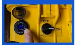
Turn on all units (2, 3 or 4) and check voltage display is 'on'. If below 11.8V, unit(s) must be charged.\* All units will run through the set up process and move 3 times.
